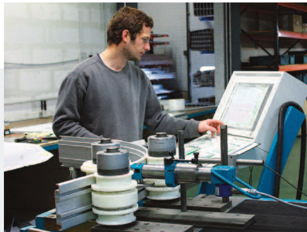
Curve production by digital bending
